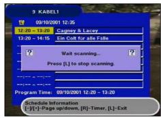
With the (G) and (F) buttons, you receive the programme overview of the currently received transmitter with time and duration (see on-screen display), provided that they broadcast the electronic programme guide (EPG).
